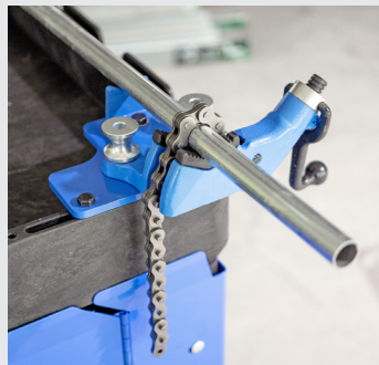
Optional 2-1/2" Bench Chain Vise mounts seamlessly
